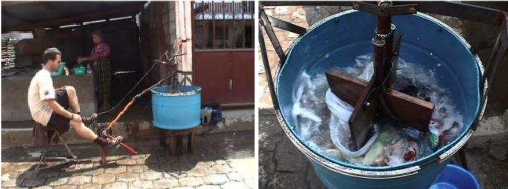
Figure 2: MayaPedal's prototype washing machine shows that demand exists, but it is difficult to use and it damages clothing.
