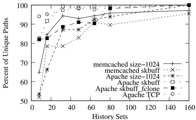
**Figure 4.** Percent of unique paths captured as a function of history sets collected. For all data types, the maximum number of unique paths is based on a profile with 720 history set. Only results for profiles with less than 160 sets are shown.
