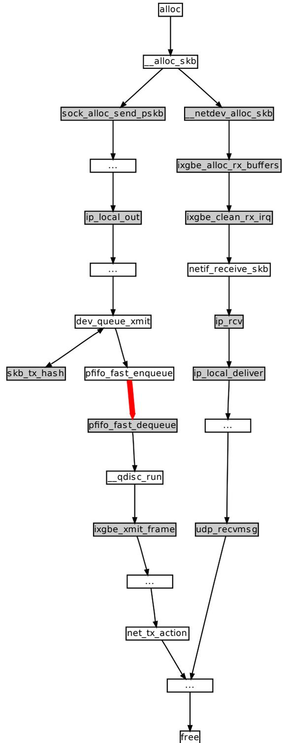
**Figure 2.** Partial data flow view for `skbuff` objects in memcached as reported by DProf. The thick line indicates a transition from one core to another. Darker boxes represent functions with high cache access latencies.
