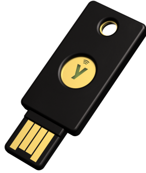
Figure 2-2: The YubiKey, the most popular commercial FIDO2 security key, comes in a small USB-stick form factor and supports USB and NFC protocols for use with PCs and mobile devices.
